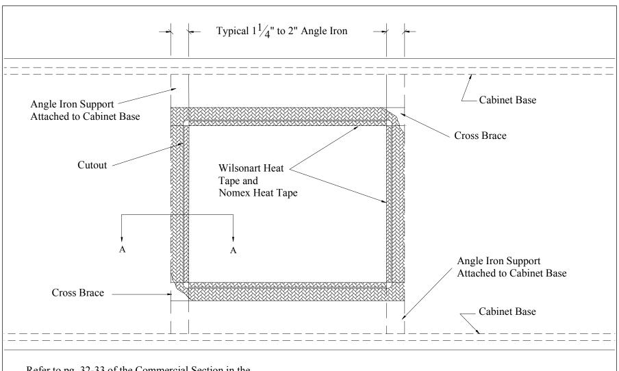
Refer to pg. 32-33 of the Commercial Section in the Gibraltar Fabrication Manual for cutout requirements
